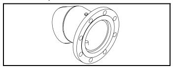
**One-pass evaporator** provides a lower pressure drop through the evaporator for applications with low delta T (temperature) or high flow or where the evaporators are piped in a series or side stream arrangement. One-pass evaporator is only available with flanged connections and with discharge end leaving water connection.
